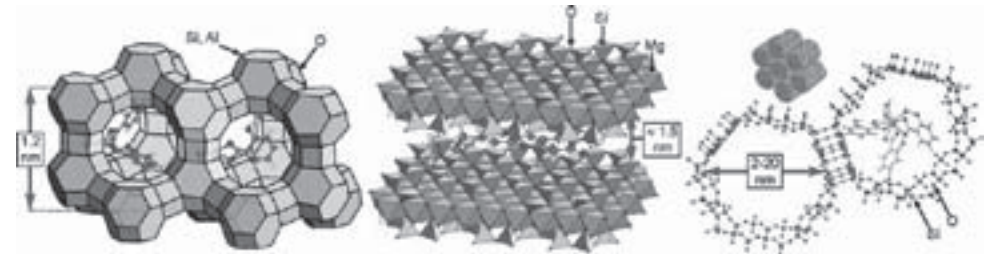
Figure 1. Left: complex (salicylate) functionalized zeolite X. Center: layered nano-silicate carrying an organic guest ("Laponite", Nile Red). Right: Mesoporous host with channel structure (e.g. MCM 41) with an embedded metallo-organic complex (salicylate).
